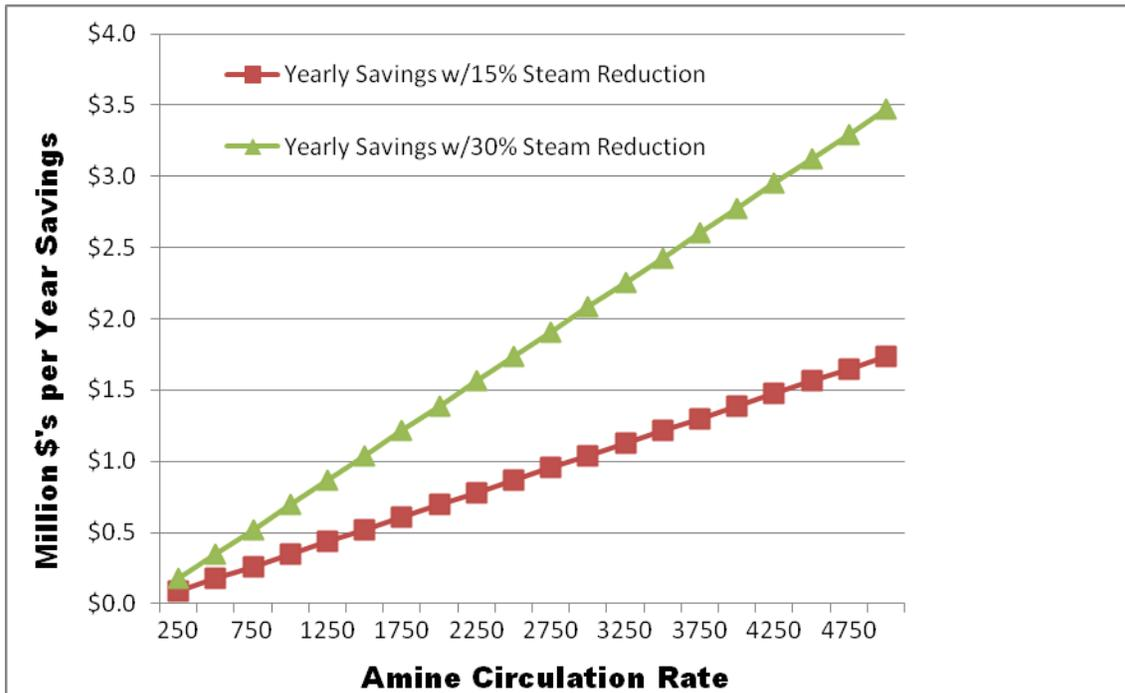
In summary, high levels of HSAS are not desirable in amine systems and can be the source of various operational and mechanical problems. However, maintaining low to moderate levels of HSAS in your amine system can provide significant energy savings. Therefore, proper management of HSAS in an amine system is essential and can yield tremendous benefits by avoiding problems while capitalizing on the available energy savings.
