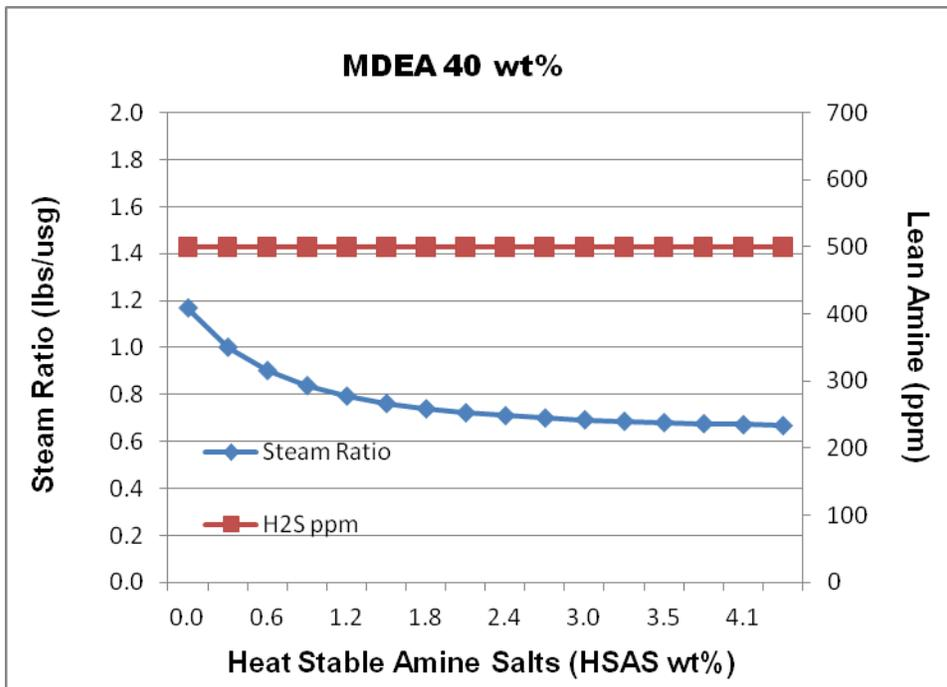
High levels of HSAS can wreak havoc on your amine system, resulting in corrosion, foaming, inability to obtain spec gas and over-stripping but steam energy savings may be a benefit from maintaining a low to moderate level of HSAS in your system. In Figures 7
