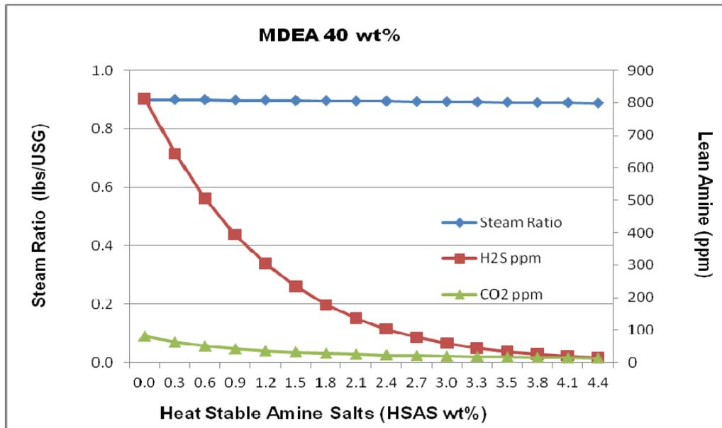
Since it is more energy efficient to regenerate an amine solution with a high level of HSAS, why don't we let them build-up to 5-10%? One answer is immediately obvious: HSAS are corrosive and at high levels they can result in pitting, metal loss and ultimately leaks and failures. High levels of HSAS can also cause foaming issues and can limit absorber performance in cases where the absorber performance is nearing maximum load of the amine.
