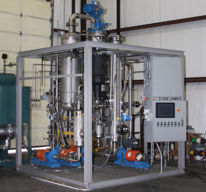
Portable "Mini" Short Path Distillation System - Hartland Distillations, Inc. - Evansville, IN
